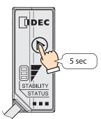
The indicator LEDs (green/orange/red) will all flash (2 seconds on, 2 seconds off) and the unit switches to maintenance mode.
