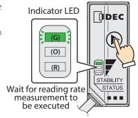
The indicator LED (orange) will flash and the unit will switch to the waiting state for measurement of the reading number of times to be executed.
