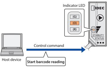
Method 3 Turn on the external trigger input.
