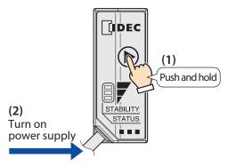
**2** Push the Operation button until you can confirm the indicator LEDs (green/orange/red) have flashed. (Approximately 5 seconds or longer)
