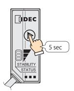
The indicator LEDs (green/orange/red) will flash and the unit will switch to the waiting state for measurement item to be selected in setup support mode.
