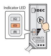
Method 2 Input the "start barcode reading" control command.
