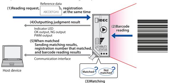
Reference data can be input with control commands. For details, refer to "5. 5 Control commands list" - P. 5-6 "Start matching".
