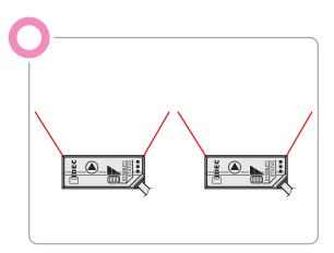
• Install the WB1F so that two or more barcodes do not enter the reading area. The WB1F cannot simultaneously read multiple barcodes.
