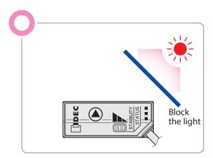
• Do not install a reflective body (metal or mirror) along the light receiving axis.
