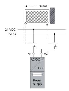
Use the same wiring logic for 24 VAC supply.
