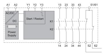
A connection in series can be used, for example, to implement a non-safety-related diagnostics function that provides feedback to other equipment while the safety-related function uses one or several of the normally open relay contacts.
