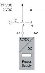
Use the same wiring logic for 24 VAC supply.
