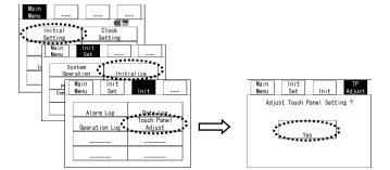
(3) Press the center of the X mark, then the position of the mark changes one after another. Press five marks sequentially.
