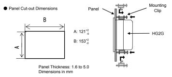
Place the HG2G in a panel cut-out and fasten with the attached mounting clips at four places of the top and bottom side to a specified torque of 0.2 to 0.3 N·m uniformly.
