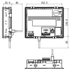
Depending on the type of connection cable used the dimensions shown above will change. The dimensions given here are representative values and are intended for reference only.
