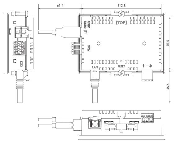
Depending on the type of connection cable used the dimensions shown above will change. The dimensions given here are representative values and are intended for reference only.
