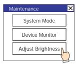
2 Press the << and >> at the bottom the Adjust Brightness Screen to adjust the contrast to the optimal setting.
